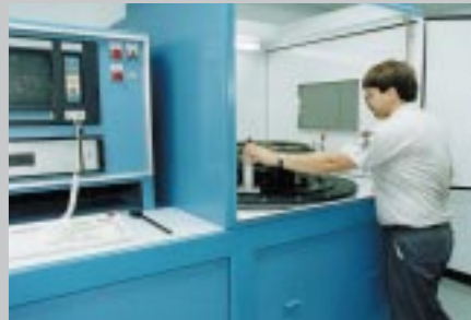
Engine Specialist Jeff Schwabke prepares a Garrett 731 turbine nozzle for analysis on Duncan's A4/A5 nozzle flow bench.
